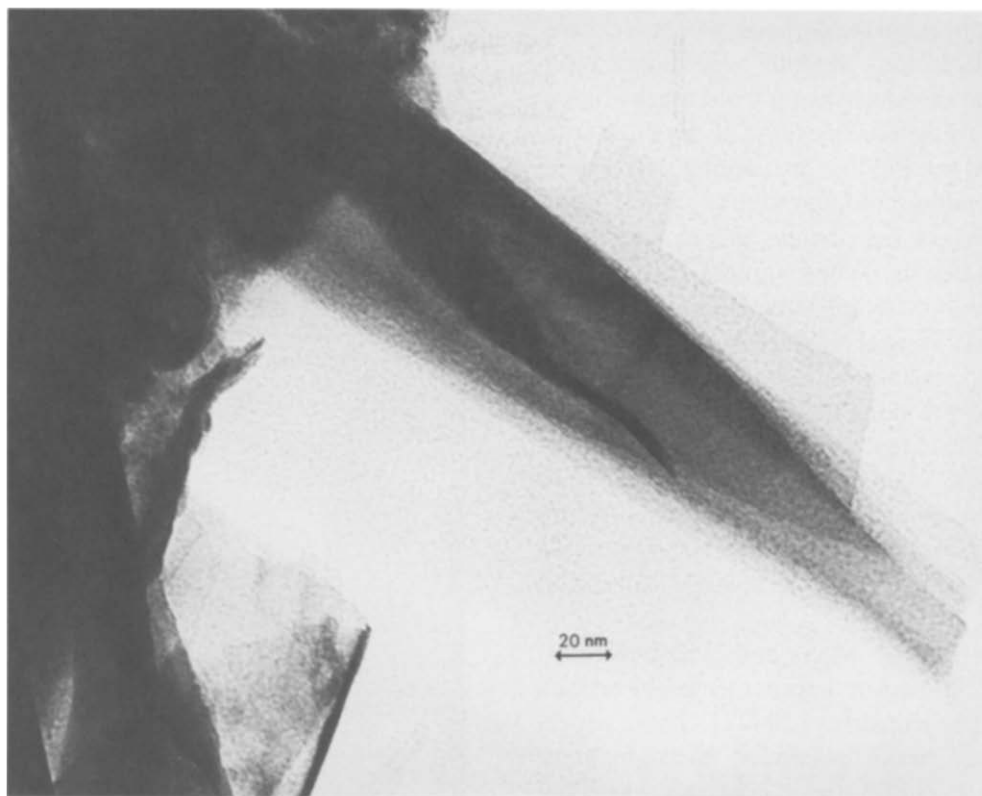
Fig. 7. TEM of \text{MoS}_2 showing 'roll' structure of layers. Note single layer of \text{MoS}_2 folded over on itself (from ref. [18]).
